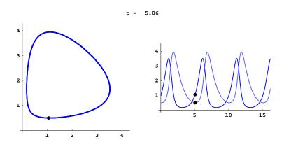
The solution shown above corresponds to the initial condition  $(R_0, F_0) = (1, 0.5)$  with parameter values a = 2, b = 1.2, c = 1, and d = 0.9. See the web site for the entire animation and for a related 3D animation. DETools also has a tool called PredatorPrey.
