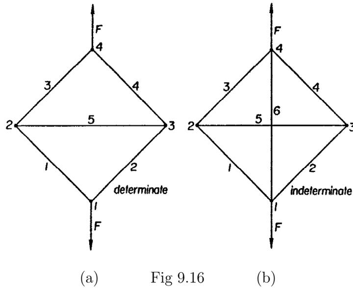
at the four nodes are as shown in Fig.9.17. For the truss of Fig.9.16(a) we obtain from equilibrium at point 1 (or equally well point 4) that  $F_1 = \sqrt{2}/F$ , and from equilibrium at point 2 (or equally well point 3) that  $F_2 = F$ , and all unknown internal forces are thus determined for truss 9.16(a). Truss 9.16(b) includes the extra unknown  $F_3$ , exerted on nodes 1 and 4 by rod 6, but there are only two equations of equilibrium, and the three  $F_1, F_2, F_3$  cannot be determined.
