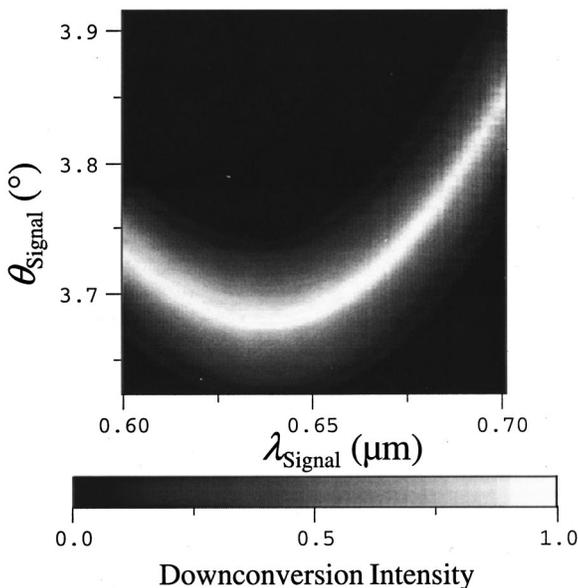
**Fig. 12** Plot for  $\Phi = f(\lambda_{\text{signal}}, \theta_{\text{signal}})$  for a KDP crystal (5-mm crystal length and 2-mm pump width) with  $\lambda_{\text{pump}}=0.351 \mu\text{m}$ ,  $\theta_{\text{pump}}=52 \text{ deg}$ ,  $\varphi_{\text{signal}}=0 \text{ deg}$ . (Here  $\theta_{\text{signal}}$  is an external angle.)
