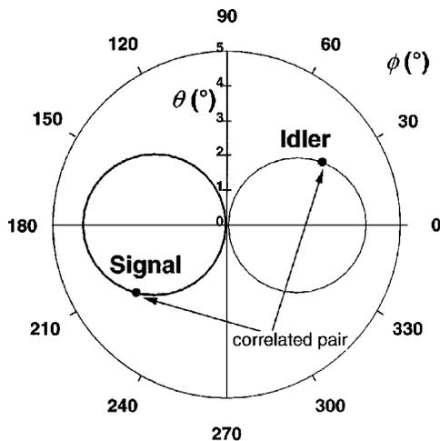
**Fig. 9** Polar plot of the direction of signal and idler output photons ( $\lambda_{\text{signal, idler}}=0.702 \mu\text{m}$ ) for  $\theta_{\text{pump}}=49.2 \text{ deg}$  and  $\lambda_{\text{pump}}=0.351 \mu\text{m}$  from a BBO crystal. The pump beam propagates out of the page at the origin.
