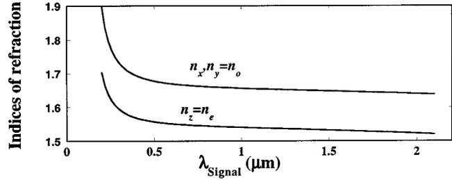
**Fig. 4** Indices of refraction versus wavelength for BBO, a negative uniaxial crystal. The graph indicates that “extraordinary” waves (polarized parallel to the optical axis  $z$ ) travel faster than “ordinary” waves (polarized transverse to this axis).
