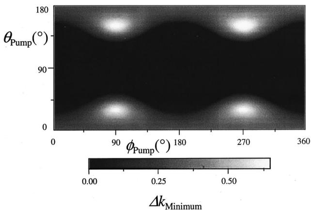
**Fig. 6** Graph of  $|\Delta \mathbf{k}|$  versus  $\theta_{\text{pump}}$  and  $\varphi_{\text{pump}}$  in a  $\text{KNbO}_3$  crystal with  $\lambda_{\text{pump}} = 0.633 \mu\text{m}$  and  $\lambda_{\text{signal}} = 0.950 \mu\text{m}$ .
