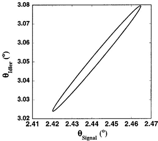
**Fig. 8** Graph of  $\theta_{\text{idler}}$  versus  $\theta_{\text{signal}}$  ( $\Phi=0.5$ ) for a KDP crystal (5-mm crystal length and 2-mm pump width) with  $\lambda_{\text{pump}}=0.351 \mu\text{m}$ ,  $\varphi_{\text{pump}}=0 \text{ deg}$ ,  $\theta_{\text{pump}}=52 \text{ deg}$ ,  $\lambda_{\text{signal}}=0.633 \mu\text{m}$ , and  $\varphi_{\text{signal}}=0 \text{ deg}$ .
