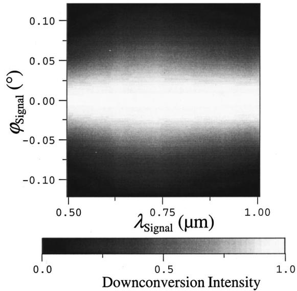
**Fig. 13** Graph of  $\Phi = f(\lambda_{\text{signal}}, \varphi_{\text{signal}})$  for a KDP crystal (5-mm crystal length and 2-mm pump width) with  $\lambda_{\text{pump}}=0.351 \mu\text{m}$ ,  $\theta_{\text{pump}}=52 \text{ deg}$ , and  $\varphi_{\text{signal}}=0 \text{ deg}$ .
