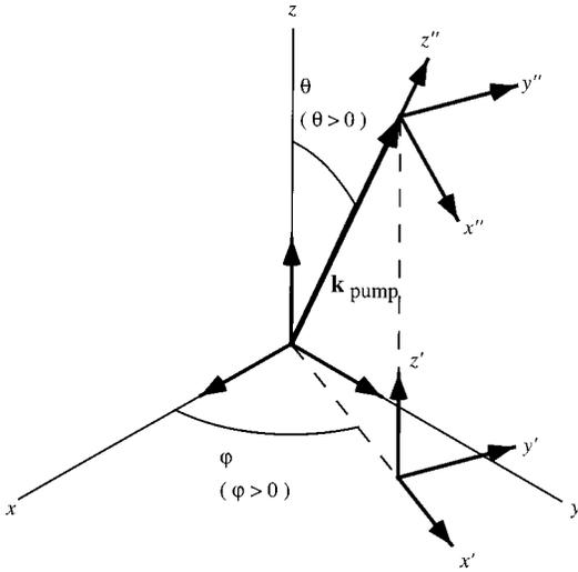
**Fig. 1** Crystal axes and the laboratory frame axes  $(x, y, z)$ , are crystal dielectric axes (the optical plane is the  $x$ - $z$  plane and  $n_z > n_y > n_x$ );  $(x', y', z')$ , rotated axes (rotation angle  $\varphi$ , about the axis  $z$ ); and  $(x'', y'', z'')$ , laboratory frame axes (rotation angle  $\varphi$ , about the axis  $y'$ ).
