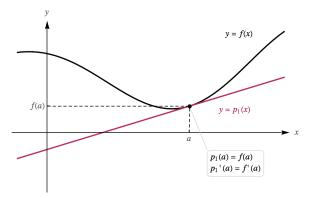
Linear approximation works well if f has a fairly constant slope near a. However, if f has a lot of curvature near a, then the tangent line may not provide an accurate approximation. To remedy this situation, we create a quadratic approximating polynomial by adding one new term to the linear polynomial. Denoting this new polynomial  $p_2$ , we let
