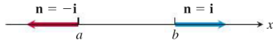
FIGURE 16.81 The outward unit normals at the boundary of [a, b] in one-dimensional space.
