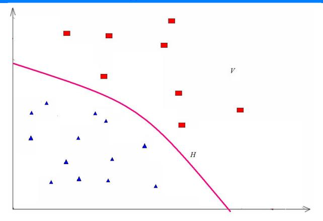
Fig. 1. Red points have y = +1 and blue have y = -1 in the space *F*.  $H : f(\mathbf{x}) = 0$  is the separating surface.
